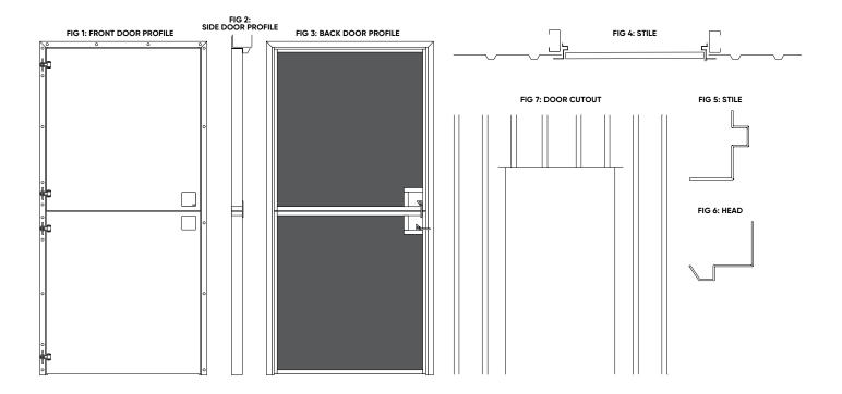
The Sentry<sup>™</sup> 801.47.1100 stable door is a metal-clad door, comprising of RHS frame with a steel skin and internal 18mm black ply cladding, pre-hung into a 47 series 3-sided jamb.
